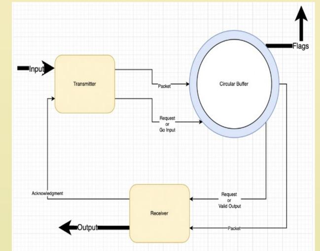
All of the components of module are connected in the given manner such that transmitter is connected to circular buffer, and circular buffer itself is connected to the receiver, and receiver is return is connected to the transmitter itself. In general, our whole module has 3 inputs and 2 outputs.
