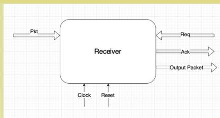
Receiver has 4 inputs and 2 outputs. Receiver works like a state machine, states will change depending on Pkt port and Req port. Clock and Reset are there just to keep this component in sync with the other component of the Module. Receiver will receive packet from Buffer and send the output to the User.
