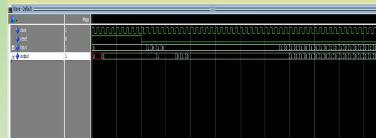
As we can see in the waveform, when the input packet is sent, after a couple of cycles we would start getting the same input packet as the output from our module. Although there is a delay in between the input and output packets.
