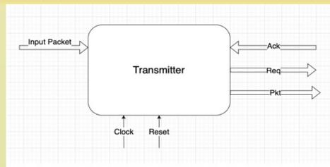
Transmitter has 4 inputs and 2 outputs. Transmitter works like a state machine, states will change depending on Input port and Ack port. Clock and Reset are there just to keep this component in sync with the other component of the Module. Transmitter will receive packet from user and send the packet to the buffer.
